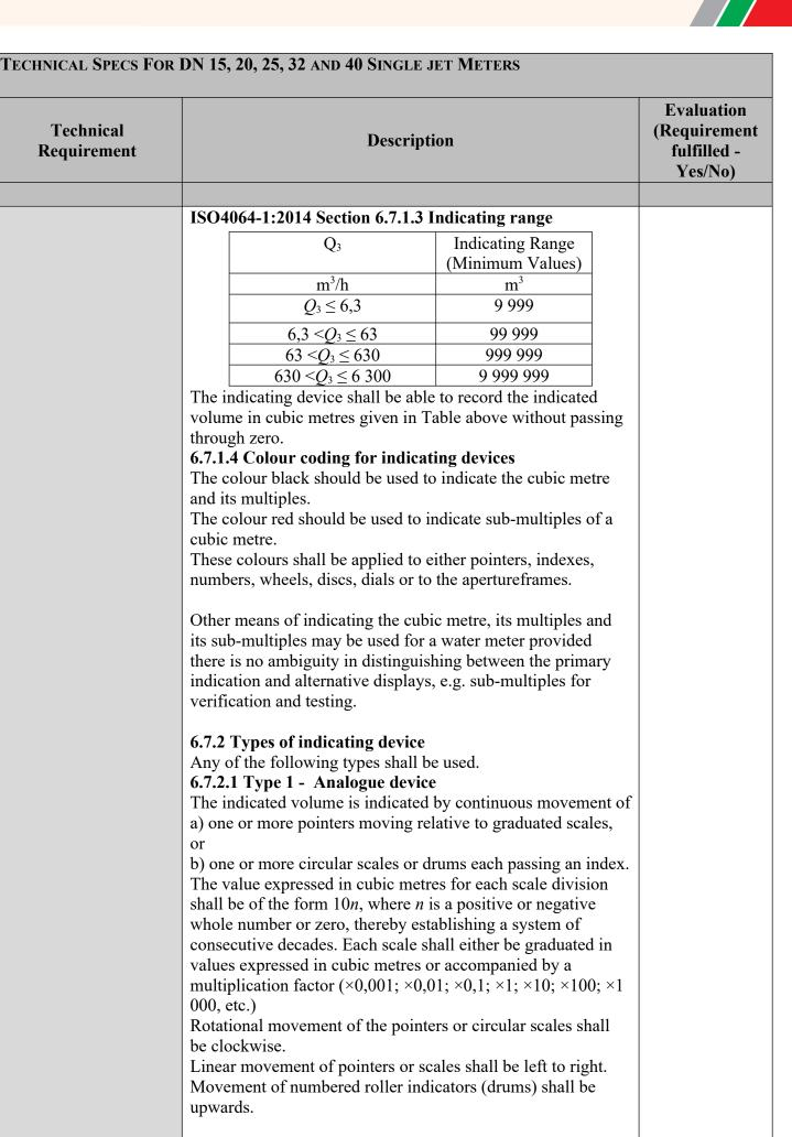
**6.7.2.2 Type 2 - Digital device** The indicated volume is given by a line of adjacent digits
