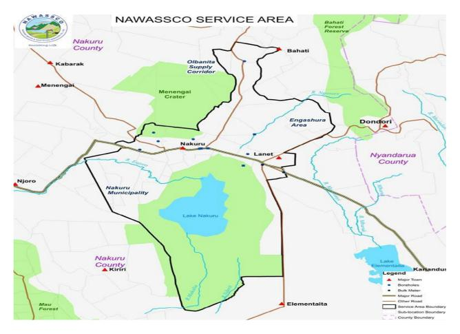
Nawassco has four Wellfield stations with fourty boreholes, two river sources and bulk water supply from Naruwasco with daily production standing at an average of 40,000m³/day against daily demand of between 70,000m³- 80,000m³. To ensure quality checks, twenty consumer sampling points have been identified where residual chlorine are checked daily before bacteriological analysis is done for quality compliance.
